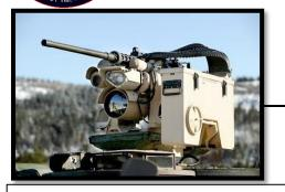
Shoot Stabilized Remote Weapon Station (RWS) - M2 Heavy Machine Gun or MK-19 Automatic Grenade Launcher - Capability to accept future weapons - 360-degree Fields of Fire
