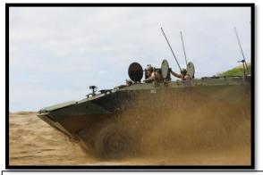
Move (Land Operations) - Cross Country Performance - Long Range / Fuel Efficient -- Negotiate 60% Slope [Front] & 30% Slope [Side] The ACV provides Expeditionary, Protected Mobility and Lift for the Marine Corps Infantry. ACV is a full replacement for the legacy AAV.
